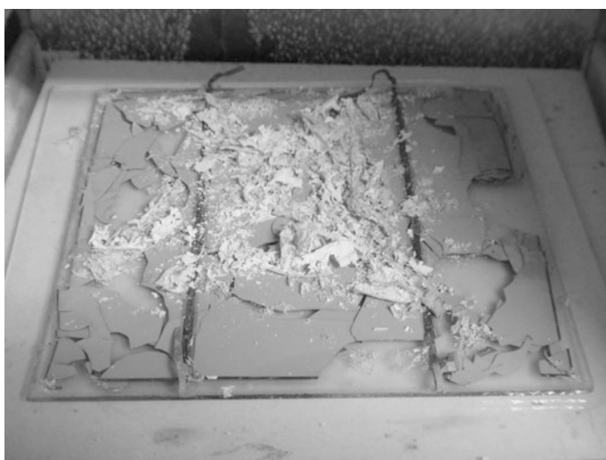
Fig. 14 Residual components of silicon module after heat decomposition
