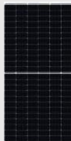
HiKu6 – CS6W-MS* Power: up to 550W Efficiency: up to 21.5% Dimension: 2261 x 1134 x 35 mm Cells: 182mm half-cut mono-PERC
